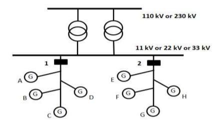
In such case, the QCA shall submit separate feeder-wise forecast at Point '1' and '2' i.e. for Intra-State and Inter-State respectively. TNSLDC shall Schedule at Point '1' being Intra-State and at State Periphery for Point '2' by applying Transmission losses as per TNERC FSDSM Regulations 2024 and its amendments.
