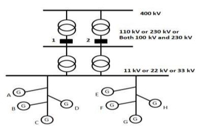
In this case, a group of generators ('A' to 'H') are connected at 11/22/33 kV level of the EHV Pooling Station through common 11/22/33 kV feeders.
