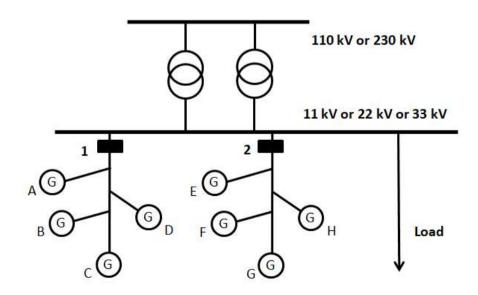
In this case, multiple generators ('A' to 'H') are connected at 11/22/33 kV level of the EHV Pooling Station through common 11/22/33 kV feeders selling power within the State.
