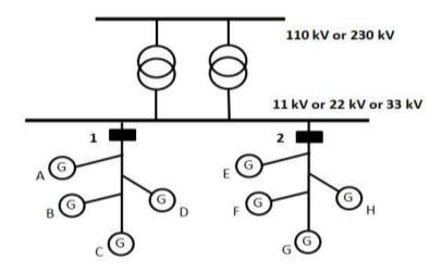
In such case, the Forecast shall be done by the QCA at Points 1 & 2 together. Scheduling and Accounting shall be done by TNSLDC at Points '1 2' together for the Pooling Substation. The QCA shall de-pool the deviation charges among respective generators separately based on the mechanism developed within themselves.
