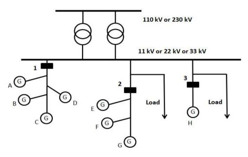
TNSLDC shall carry out scheduling and accounting at Points '1, 2 & 3' for Pooling Station as a whole and the QCA shall de-pool the deviation charges among respective generators separately based on the mechanism developed within themselves.
